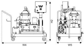
Standard module with trolley, height and width
