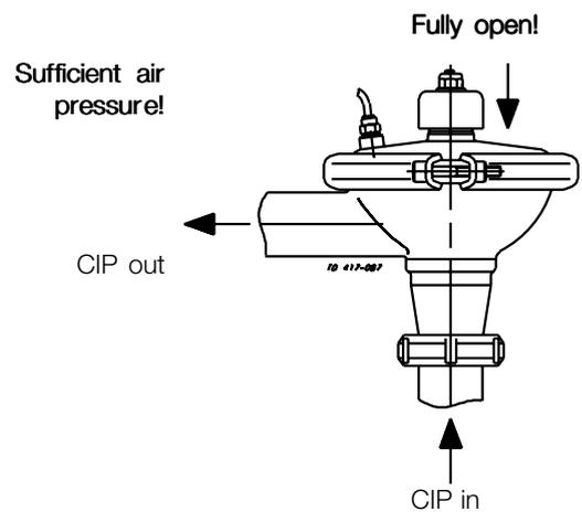
The valve is designed for cleaning in place (CIP).
