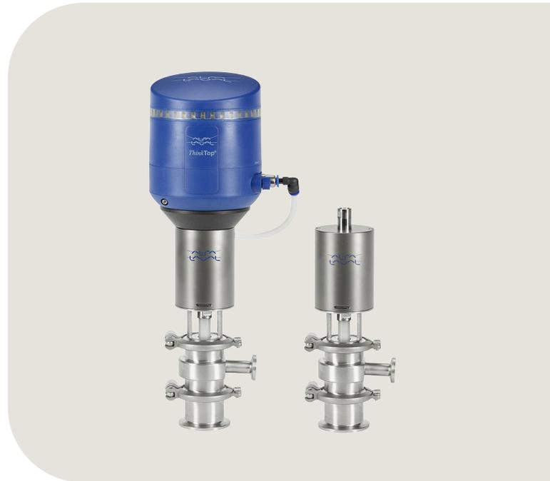
During CIP, a pneumatic actuator is used (pulsed) to force the ball off the upper seat, enabling the seat and the interior of the vacuum breaker valve to be cleaned. CIP fluid is discharged during the actuator pulse and is drained through the vent port (Fig. C).
